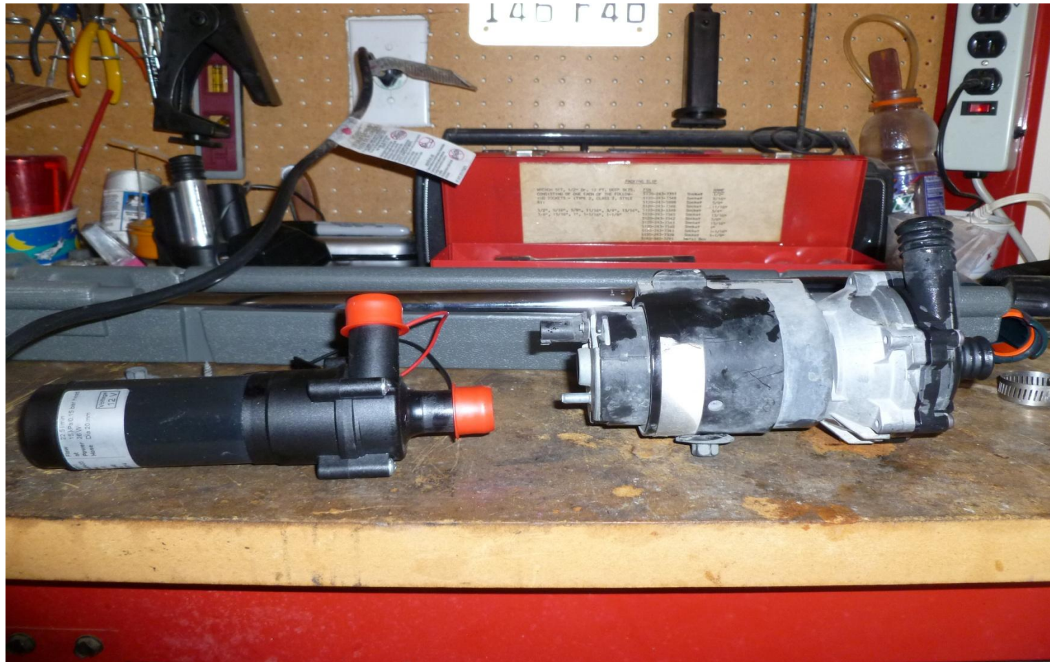
New CM30P7-1 Johnson Pump on Left, Old Bosch Pump on the right big difference in size.
