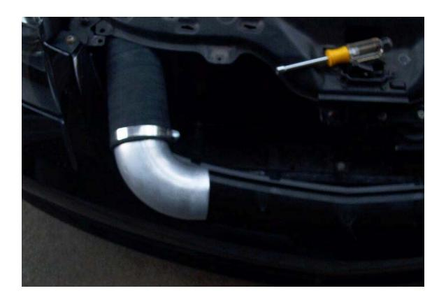
22. Once the elbow is on and secured slide the hose back towards the motor and the elbow will tuck in behind the bumper (be careful the hose clamp doesn't scratch your bumper while moving the hose).
