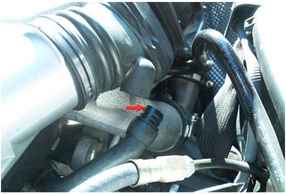
3. The main air box assembly can be taken out in one piece. Start by lifting up gently on the driver side rear of the air box to undo the bushing/clip.
