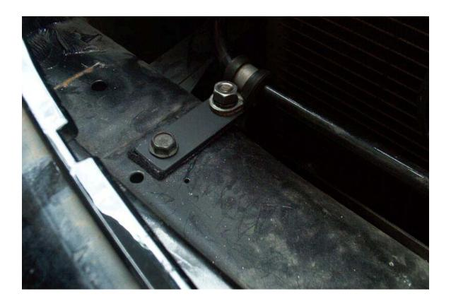
20. Insert the 13.5" long hose thru the passenger side radiator core support from the engine bay, towards front of the car. ( The hose part number should be aiming down so it won't be seen)
