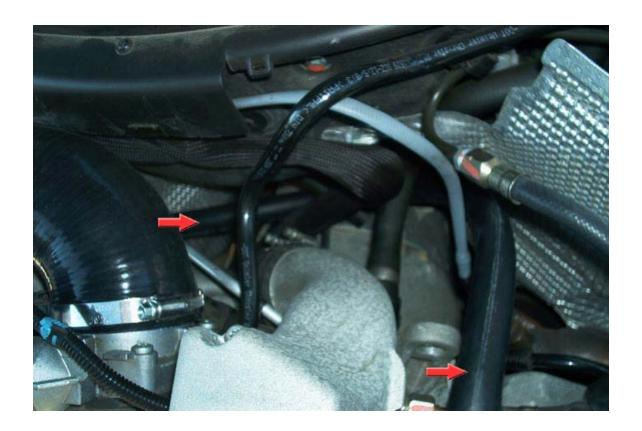
27. Attach the new intake pipe to the 90 deg coupler on the throttle body and the hose going thru the radiator support. Keep all hose clamps under the hood loose for now.
