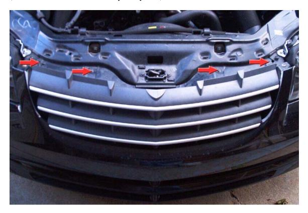
11. There are four push in clips holding the bottom of the grill to the bumper. If you gently pull the grill back you can reach in there and unclip these one at a time. Start from the driver side and work towards the passenger side.
