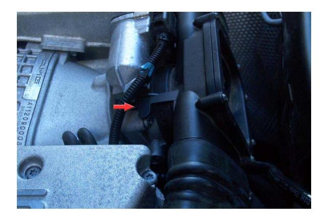
8. Once released the intake system will lift of in one piece. Gently set aside so as not to break/bend the lower throttle body clip
