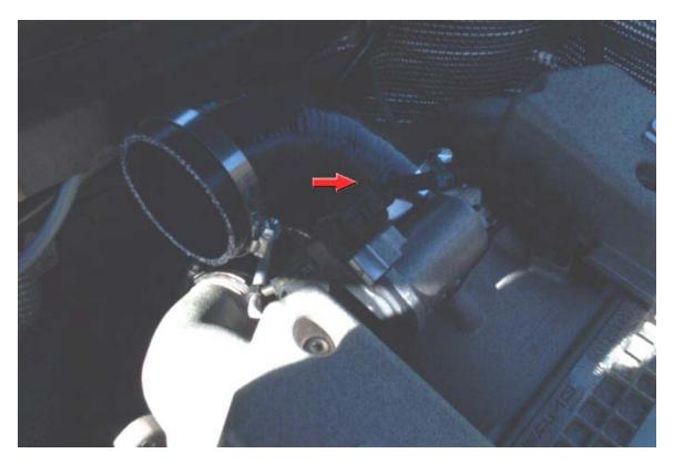
25. Attach the 27" long 3/4" hose to the port on the underside of the large intake pipe.
