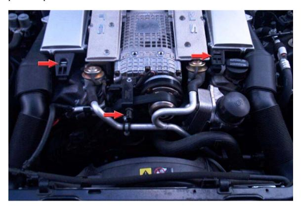
2. Disconnect the valve cover breather hose from the factory intake system (it pulls right out).
