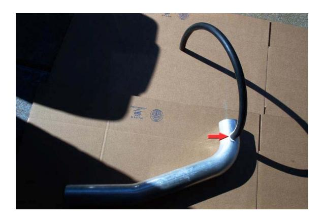
26. As the new intake is being set in route the other end of the ¾" hose behind the motor and to the valve cover port on the driver's side.
