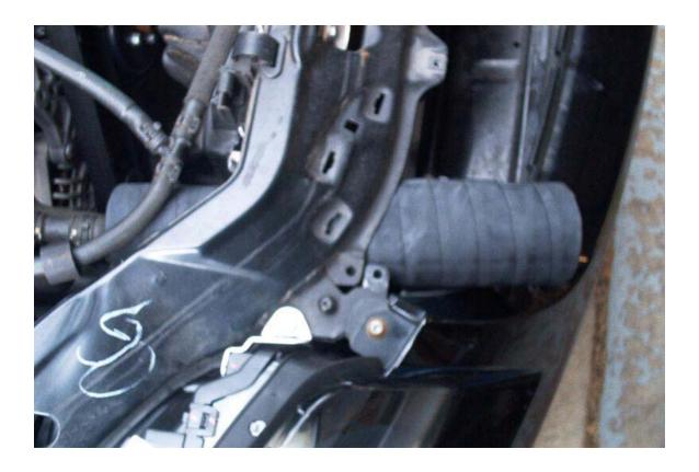
21. Pull the end of the hose past the bumper to attach the aluminum elbow and hose clamp. Have the hose clamp screw in the 2 o'clock position so it doesn't interfere later.
