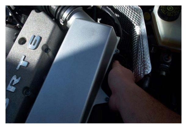
4. Next lift up on the front of the air box assembly to undo the other bushing/clip.
